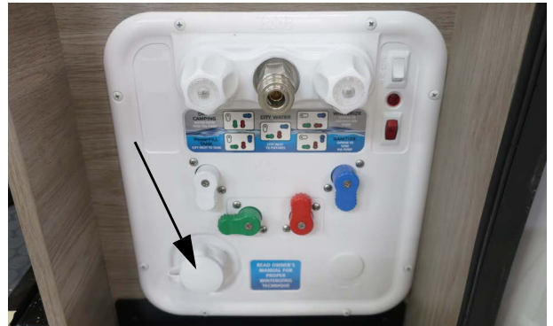
Tank Fill Inlet (Located behind the passenger rear door)
