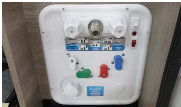
Exterior Shower/Wash Station (located behind rear passenger side door) - Typical View
