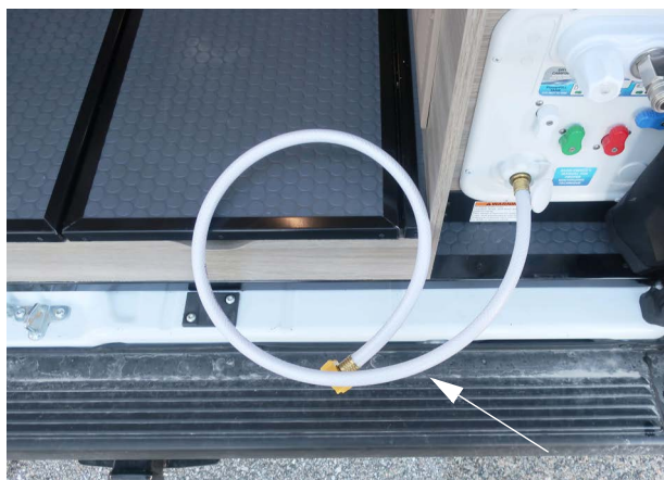
• Antifreeze Siphon Tube attached to the tank fill inlet -Typical View
