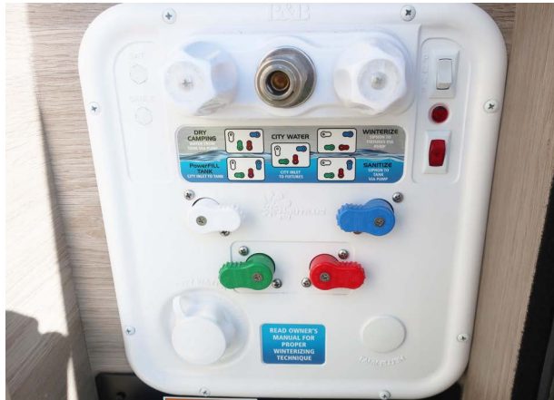
Water Center Panel in “Winterize” configuration (Panel located behind passenger rear door) -Typical View
